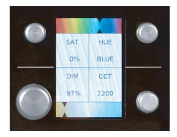
CH. 4 - Hue (H) – To optionally add saturated color, the HUE control adjusts the hue, the color of which is displayed on the control panel, or managed on the fourth DMX channel.
